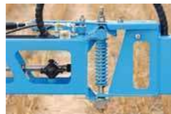
Breakaway boom ends at the front and the rear
