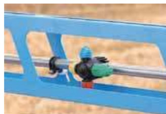
Folded metal frame with integrated spray circuit, nozzle holder and nozzles.
