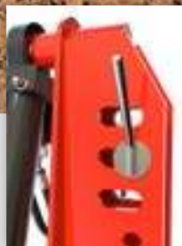
Slotted and inclined top link holes
